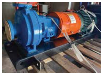
Recessed Impeller pump skid for a Summit Pump 2196R.
