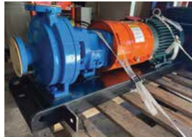
Recessed Impeller pump skid for a Summit Pump 2196R.
